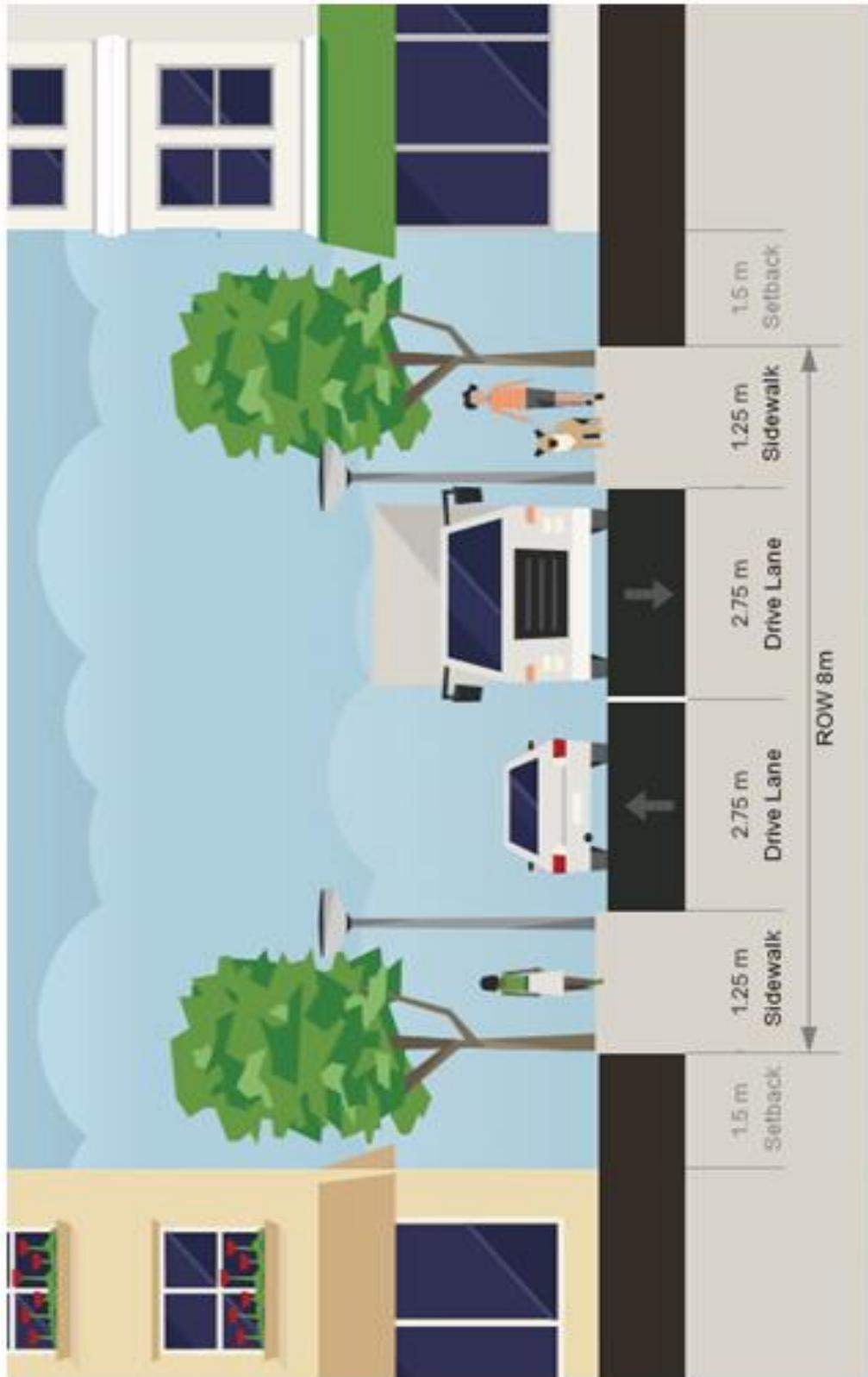
Figure 5: Cross section of a typical Class B Road
